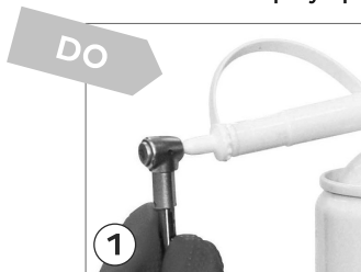
Chuck care with spray tip
