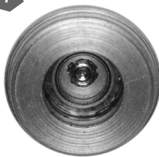
Push-button was abraded due to incorrect use
